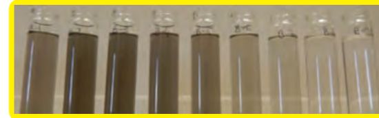
Return to the initial situation after a 9 min backwash for the sand filtration
