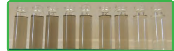
Return to the initial situation after a 6 min backwash for the GARO®filtre filtration
