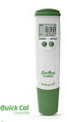
The HI-98131 is a slim, lightweight and waterproof pocket sized meter that measures pH, conductivity (EC), total dissolved solids (TDS) and temperature. All operations and settings, including calibration buffers and temperature scale selections, are made using two buttons.
