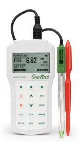
The HI-98168 is a rugged, waterproof, portable pH meter that allows for the direct measure of soil pH. This portable instrument has all the performance features of a benchtop meter. It is supplied with a specialised pH electrode that has a rugged conical tip, open junction design and a glass body making it ideal for measuring the pH of soil directly or after preparation of a soil slurry with deionised water.
